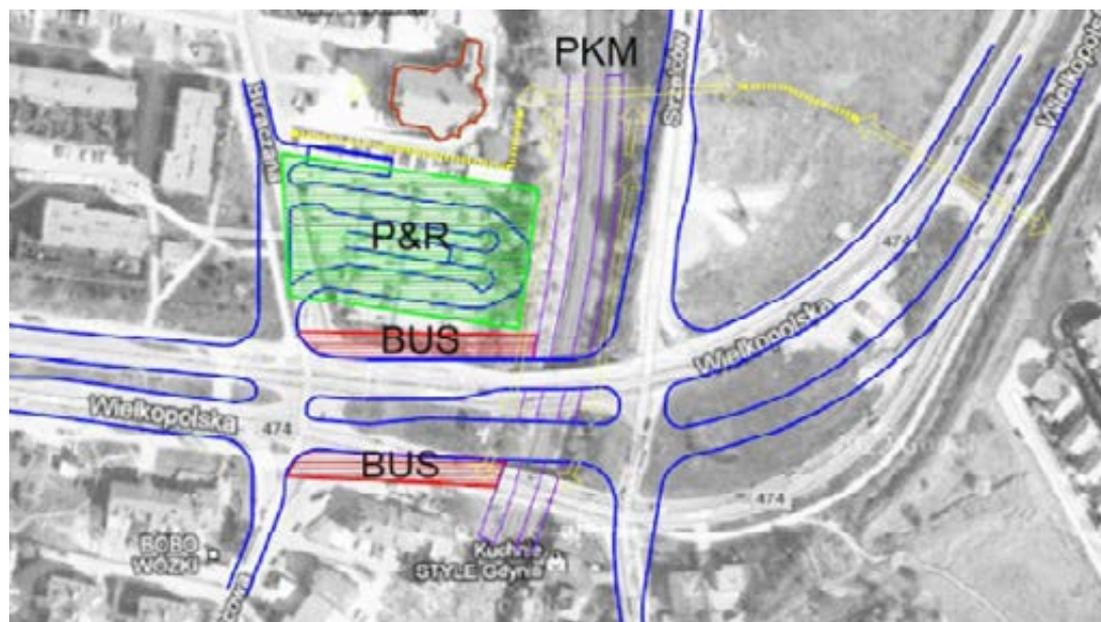
The second option is the construction of a bus/trolleybus terminus instead of a part of the parking facility. It would provide more convenient interchange but would result in a significant decrease of parking capacity (only 200 cars) and shortening/reconstructing the routes of trolleybuses and buses.
