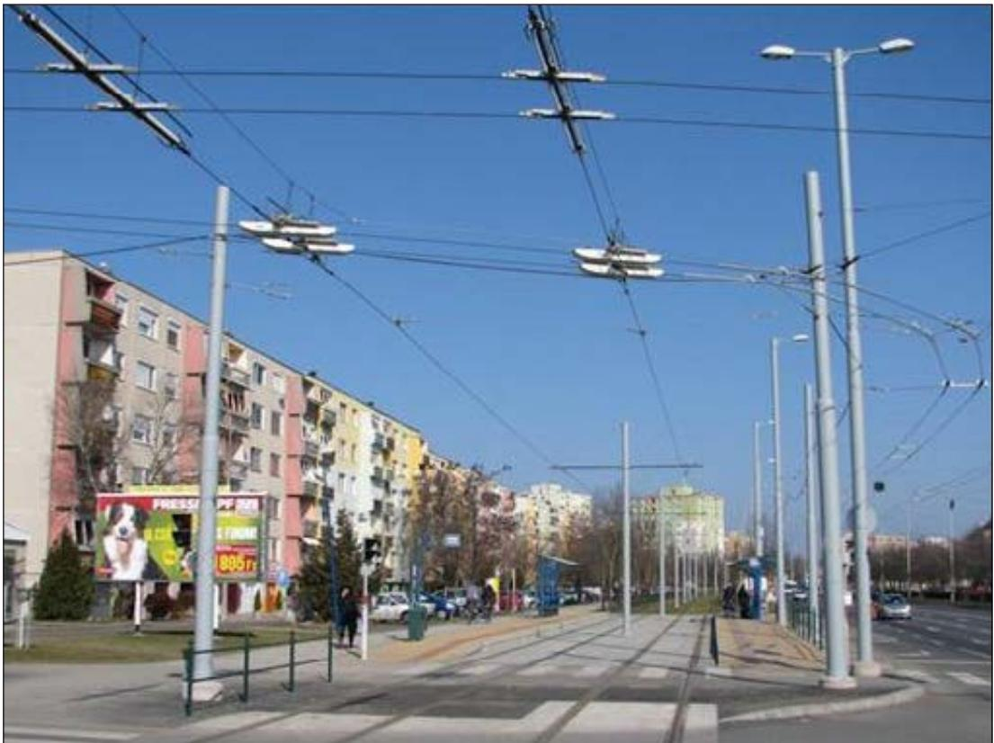
By operating a trolleybus network one needs to be aware, that if there are sub-stations in the trolleybus network that are solely used for trolleybuses, then it is likely that the “-” side of this network part is not grounded. One needs to have attention at the meeting of the grounded and the non-grounded network parts (at section insulators or e.g. at tram-trolleybus overhead crossings).
