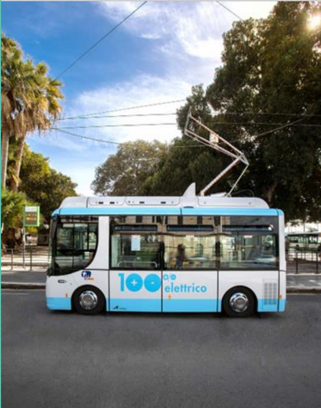
▶ In motion charging trolleybus (Cagliari)
