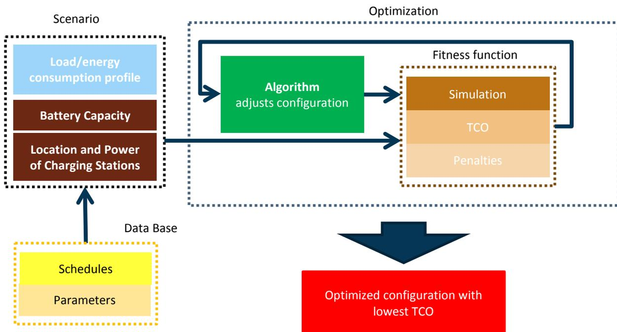
Figure 5 – Scenario calculation & optimization loop
