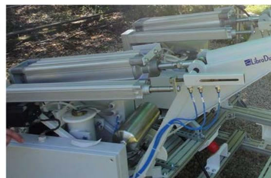
**Figure 20 – Automatic wiring system from Kummler + Matter / Dialogica**
