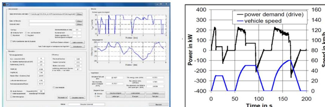
**Figure 3 – Transforming route profile into load profile**
