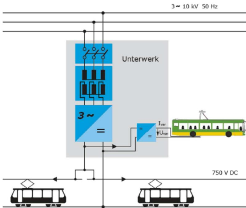
**Figure 8 – Schematic Sketch of the Bus Charging from the Tram Sub-station at the Station Neumarkt (source: Müller-Hellmann)**
