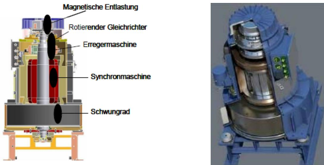
**Figure 15 – Flywheel layout examples (cross-section and 3D view)**
