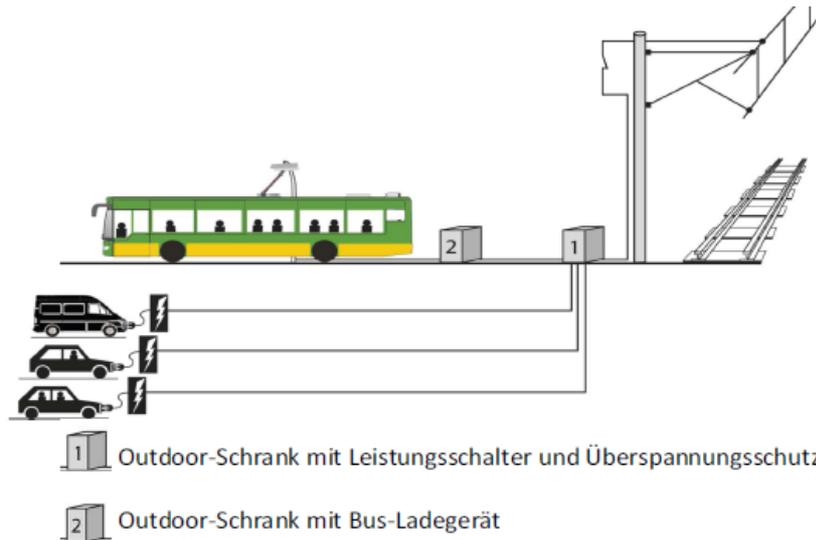
**Figure 12 - Schematic Sketch of Fast-charging for e-Vehicles from the Tram Catenary at the Train Station Sterkrade (source: Müller-Hellmann)**
