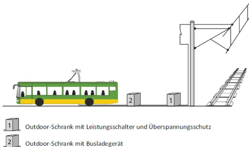
**Figure 10 – Schematic Sketch of Bus Charging from the Tram Catenary at the Train Station Sterkrade (source: Müller-Hellmann)**
