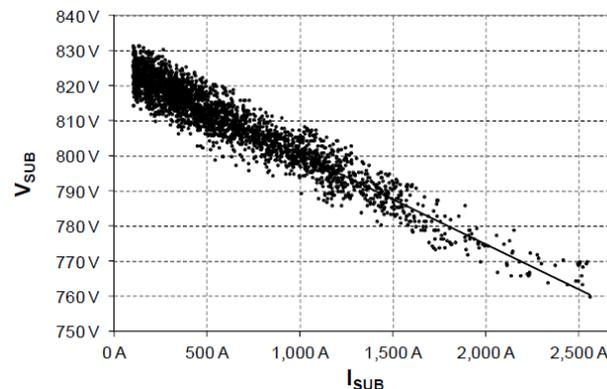
**Figure 25 - Typical Open Circuit voltage of a traction substation**
