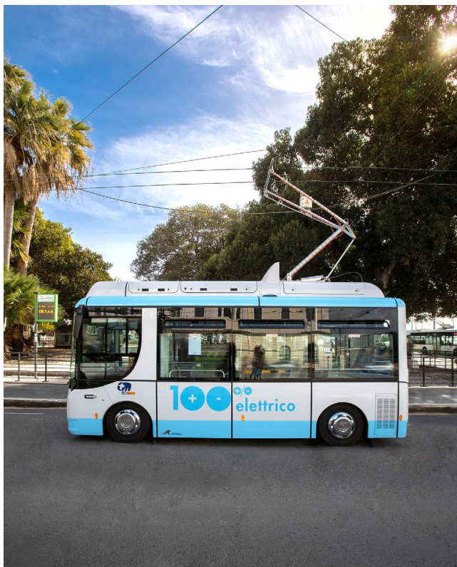
► In motion charging trolleybus (Cagliari)
