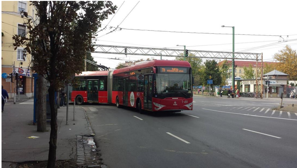
Ikarus-Škoda trolleybus (from 2013-14) the first (?) Li-ion battery trolleybus in Europe
