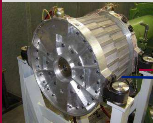
TFM as generator
