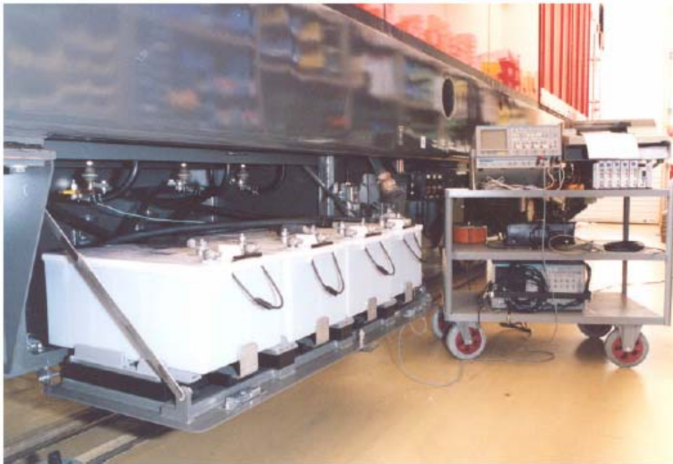
Battery compartment with lead batteries. Total weight more than 300 kg
