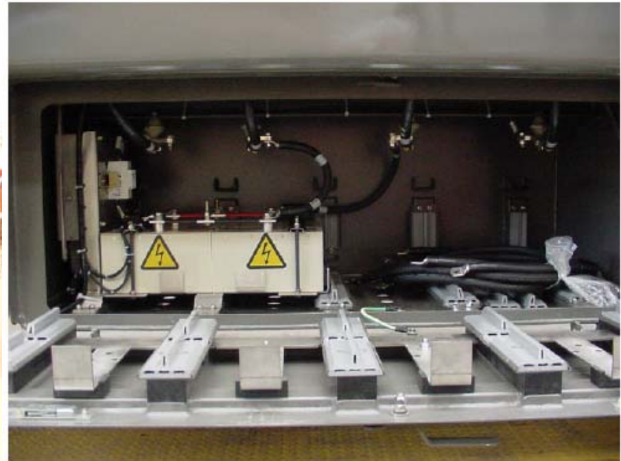
Battery compartment with Uc's module Total weight less than 30 kg
